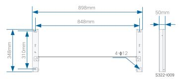
figure 4-1 Dimensions of Mounting-bracket
