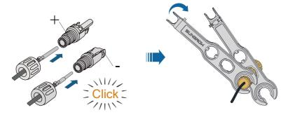
Step 4 Check for polarity correctness.
